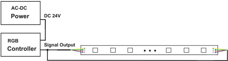
Type 2. Single Power Supply, Double Ends Feed
